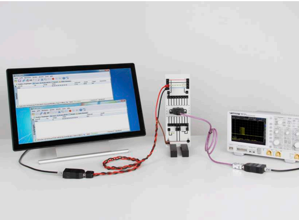
Networking automotive systems: "CAN FD databus" (A2.6.1.9)
