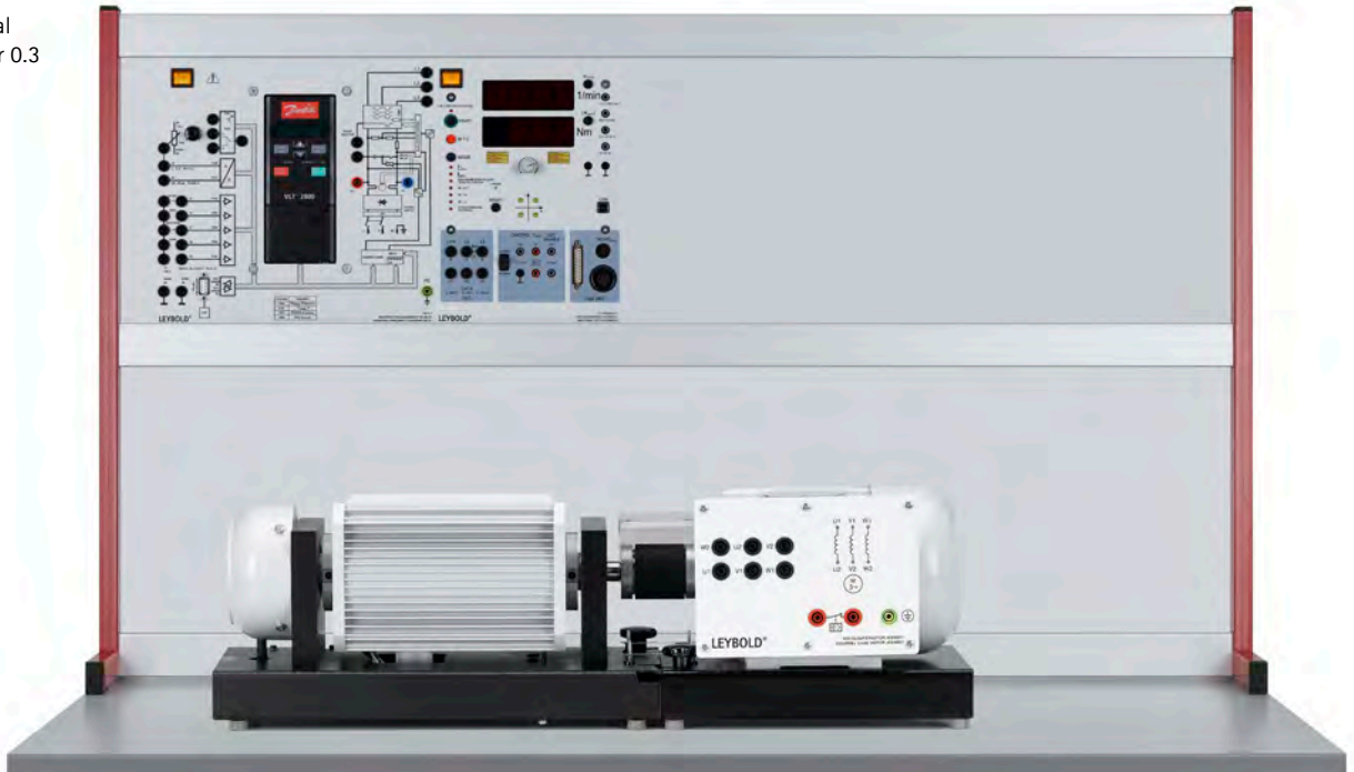
Drives with Industrial Frequency Converter 0.3 (E2.5.3.4)
