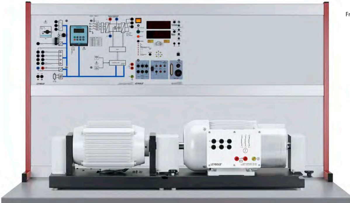
Drives with Industrial Frequency Converter 1.0 (E2.5.3.5)
