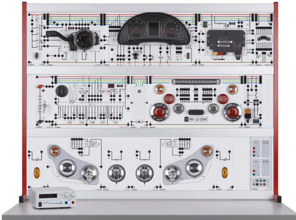
Automotive lighting with CAN data bus (A2.1.3.1)
