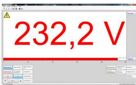
DMM high-voltage measurements with warning
